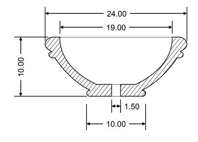
Concrete bowls are formed with fiber reinforced concrete with a water sealer additive and color all through the bowl. Cured for strength and durability.
